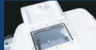
Live Bait Tank In Back Deck
