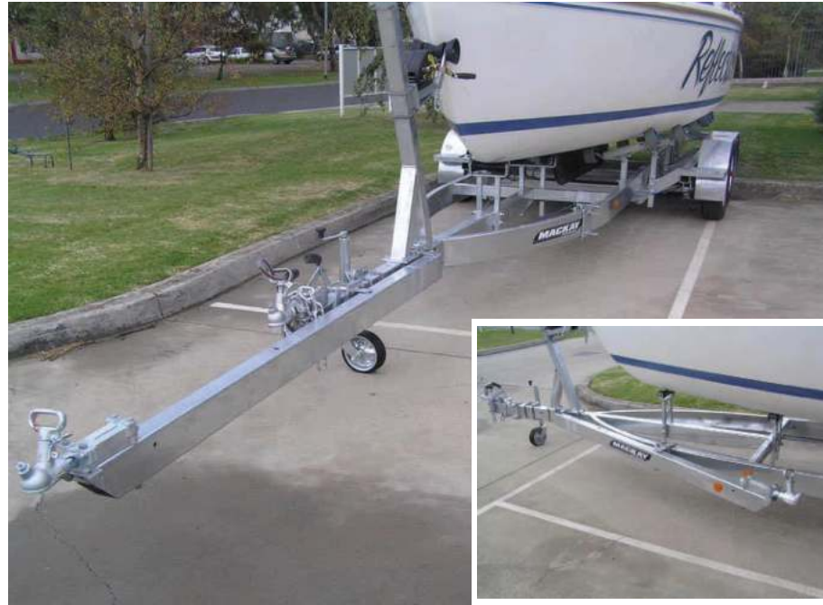
Swing Around Drawbar - Gain an EXTRA 2M
